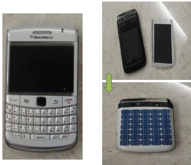
Figure 10: the efficient connection of the thin film solar cell to the mobile phone.
